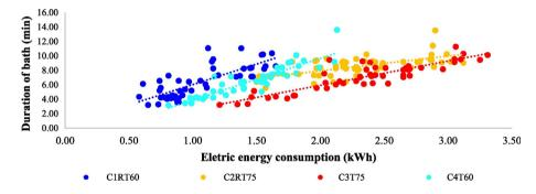
Fig. 2. Relationship between bath duration (min) and electric energy consumption (m<sup>3</sup>).
