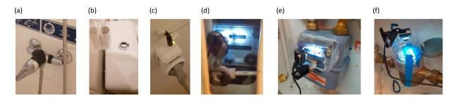
Fig. 1. Sensors: (a) Shower, (b) Flushing cistern, (c) Washing machine sensor, (d) Electricity meter, (e) Gas meter, (c) Water meter.
