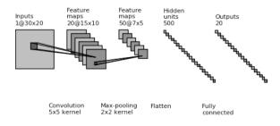
Fig. 4. Convolution neural network architecture - Read unit digits.
